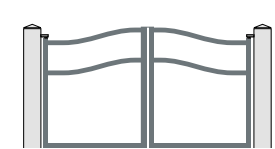
Transom in same shape for 2-leaf bowler hat- or arch- shaped gate
